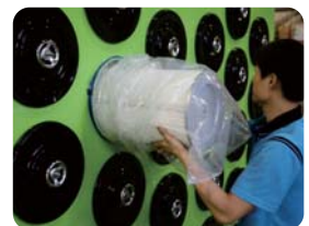
Prevent secondary contamination when changing filters
