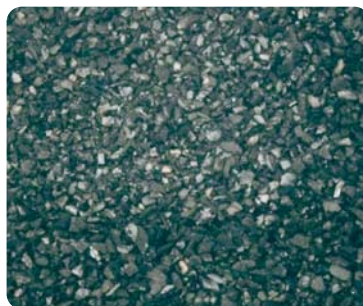
Granular activated carbon convenient recovery of absorbent matter and suitable for removing air pollutant
