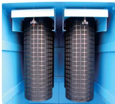
Filter structure with large filtering area
