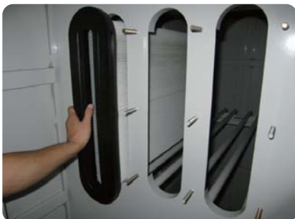
Filter system (high efficiency / easy replacement)
