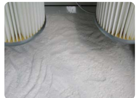
Filtering agents (Zero Power) Scatter filtering agents on the filter to prevent gluey fume adhering to the filter
