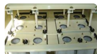
Automatic filter cleaning system (Air Pulse Jet System)
